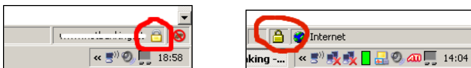
Fig. 6.8a: Symbols signalling a secure connection in Firefox and Internet Explorer Web browsers
